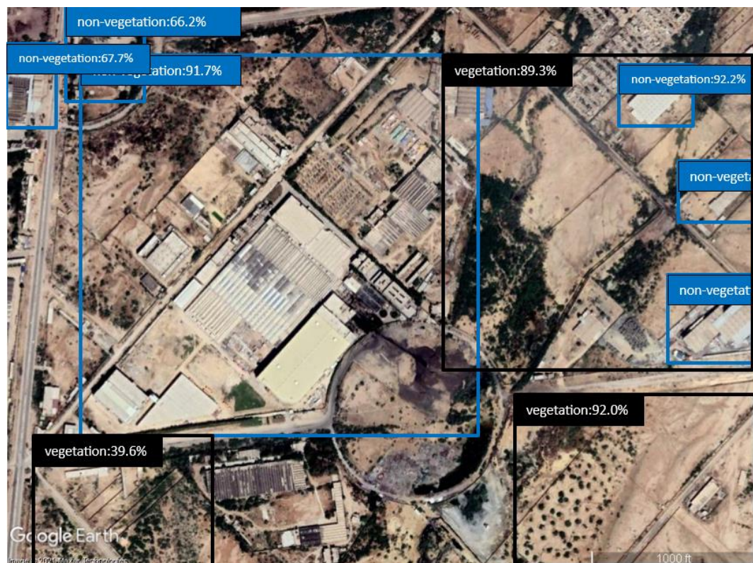
Fig. 5-g Detected areas of vegetation/ non-vegetation by the YOLOX model on the test set.
