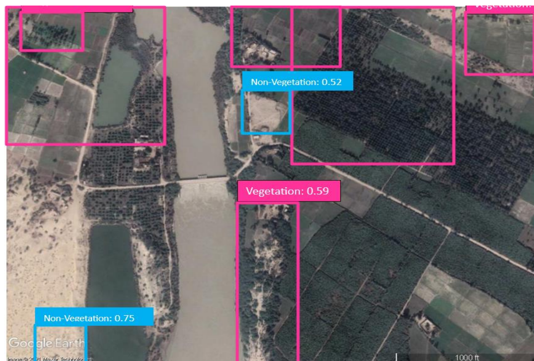
Fig. 5-f Detected areas of vegetation/ non-vegetation by the YOLOR model on the test set.
