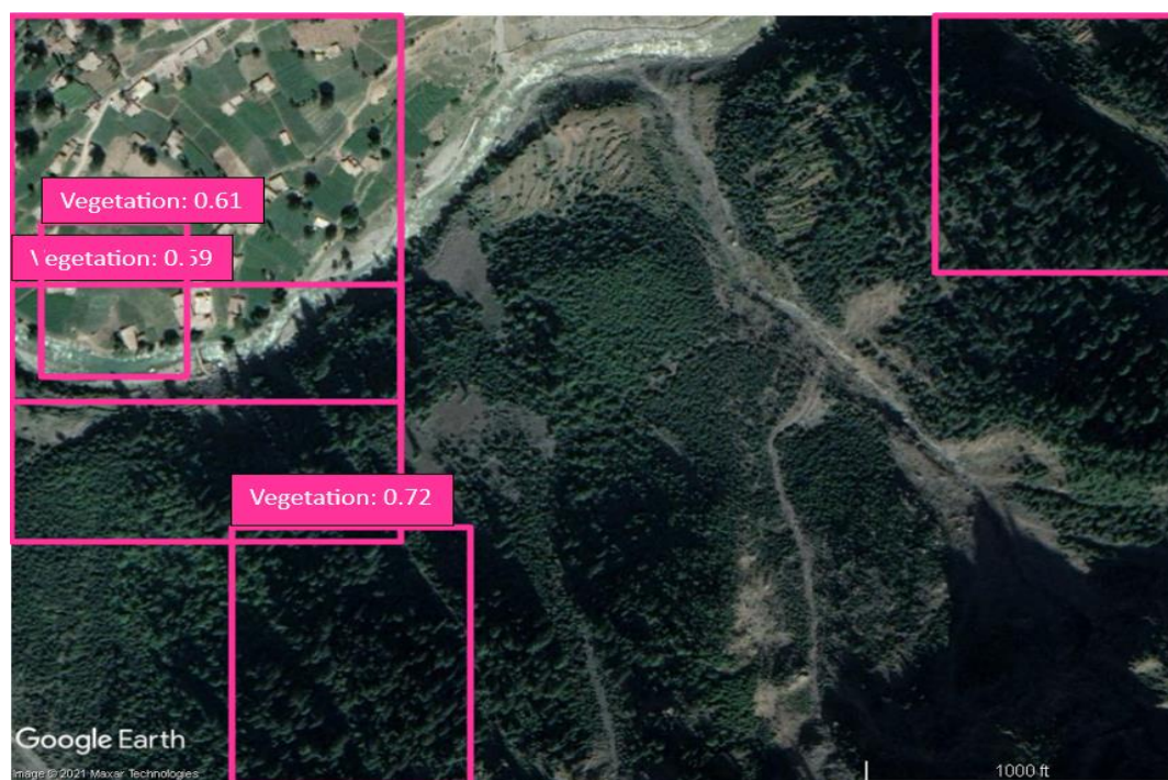
Fig. 5-h Detected areas of vegetation/ non-vegetation by the YOLOR model on the test set.
