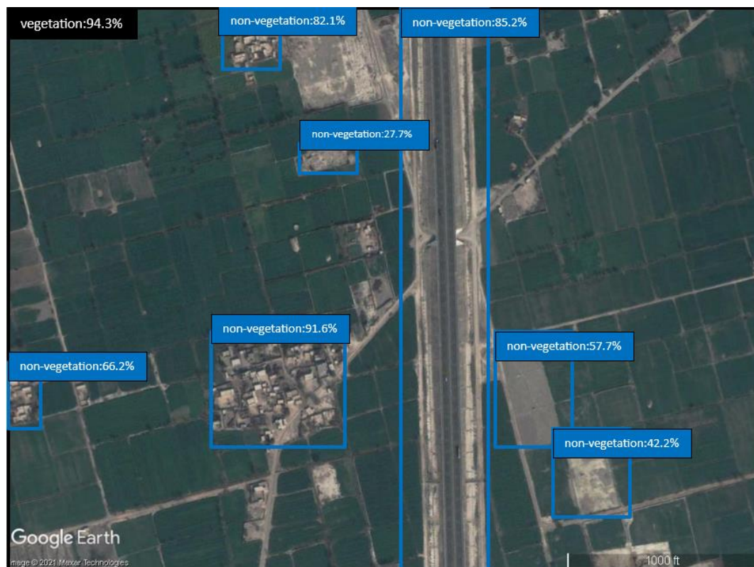
Fig. 5-e Detected areas of vegetation/ non-vegetation by the YOLOX model on the test set.
