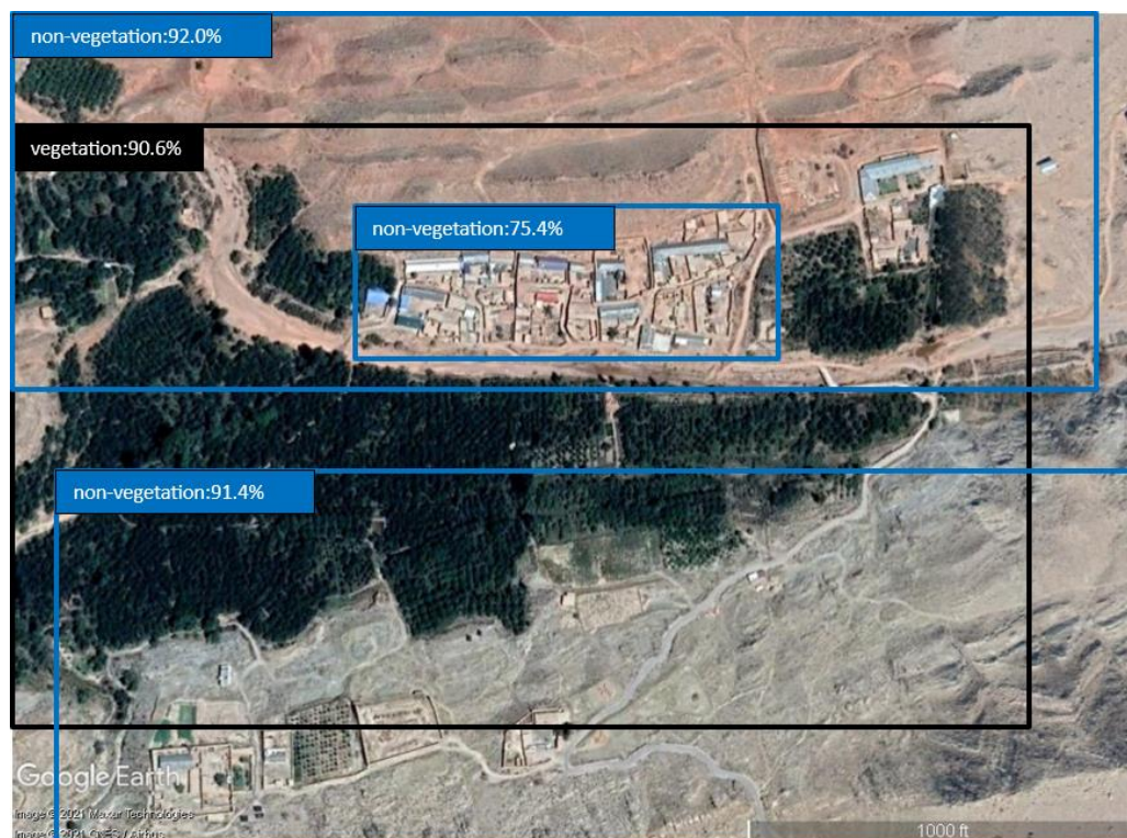
Fig. 5-a Detected areas of vegetation/ non-vegetation by the YOLOX model on the test set.
