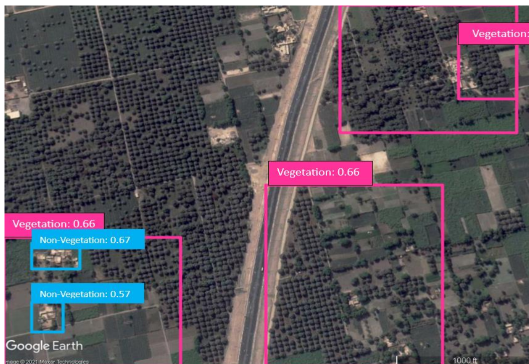
Fig. 5-d Detected areas of vegetation/ non-vegetation by the YOLOR model on test the set.
