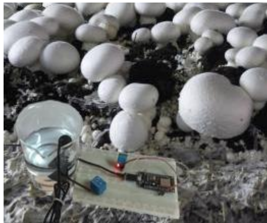
Figure 5. Internet of Things (IoT) based environment controller for mushroom cultivation.
